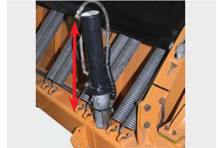
Hydraulic adjustable wheels height adjustment of the trailing wheels-solid rubber from the cabin, a double-action control unit is necessary (or switch valve)
