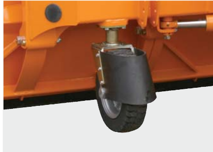
Trailing wheels-solid rubber (size II) infinitely variable through spindle, solid rubber or air tyres; Diameter 360 mm
