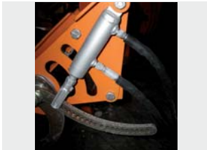
Hydraulic remote control For quantity and distance regulation from the cabin. No automatic speed adjustment.
