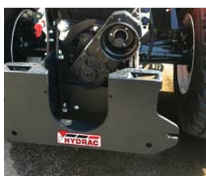
Swift transmission For use of Unimog's implements; so that the tractor's PTO remains in the same position as the unimog 1000 rpm rotation direction right side.
